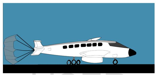
Here comes the final and the crucial stage of the LCS system. System deploys landing gear at specific altitude. At the touch down point the reverse thrusters are fired as well as the parachutes are deployed to bring the aircraft to the static position
